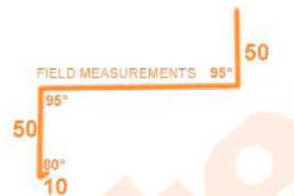
FLASHING UNDER PANEL
